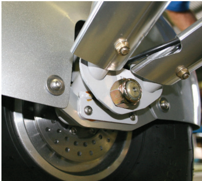
PHOTOGRAPH SHOWS INSIDE OF MOUNTED SPAT. NOTE THE ADJUSTING NUT FOR THE AXLE, REQUIRED BECAUSE THE SPAT MOUNT BRACKET MUST BE HORIZONTAL WHEN TIGHT.
