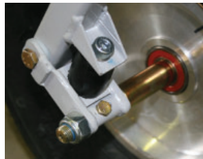
PHOTO SHOWS BOLT HEAD LOCKED AGAINST LUG
